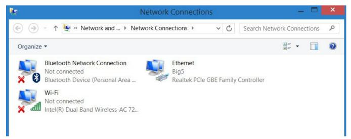
As a note the red X's above indicate that those connections are not active. Right click on the active connection and select Properties. In the next window select the Properties button Properties Disable Diagnose. A new window appears.
