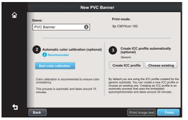
The last screen as shown on left, allows you to create your color calibration. Create ICC profile and Print test image are grayed out until you perform the Color Calibration.
