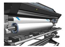
Thread the media as shown on the left, over the knurled roller. Use the roller to push the media into the machine. Once it detects media it will grab and move the media. The screen on the right appears. Select the media group and then the media name and press the Continue button.
