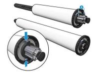
Depending on the size of the media you are loading you may need to adjust the black media stop. If the width of your roll is at the maximum width of your printer slide it to the far outside edge by pressing the two blue tabs and sliding it. If the roll width is shorter than your printers maximum width slide it in. There are a set of holes that the pins drop in from the release tabs.
