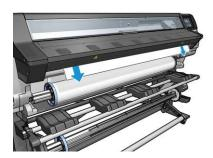
The printer will start the load process. Moving the media back and forth, checking the width and skew. If you were successful the screen on the right appears.
